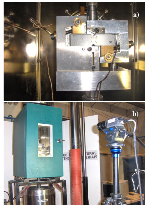
Fig. 3: Details of the test setup: a) test fixture and thermocouples; b) thermal chamber and video extensometer.
